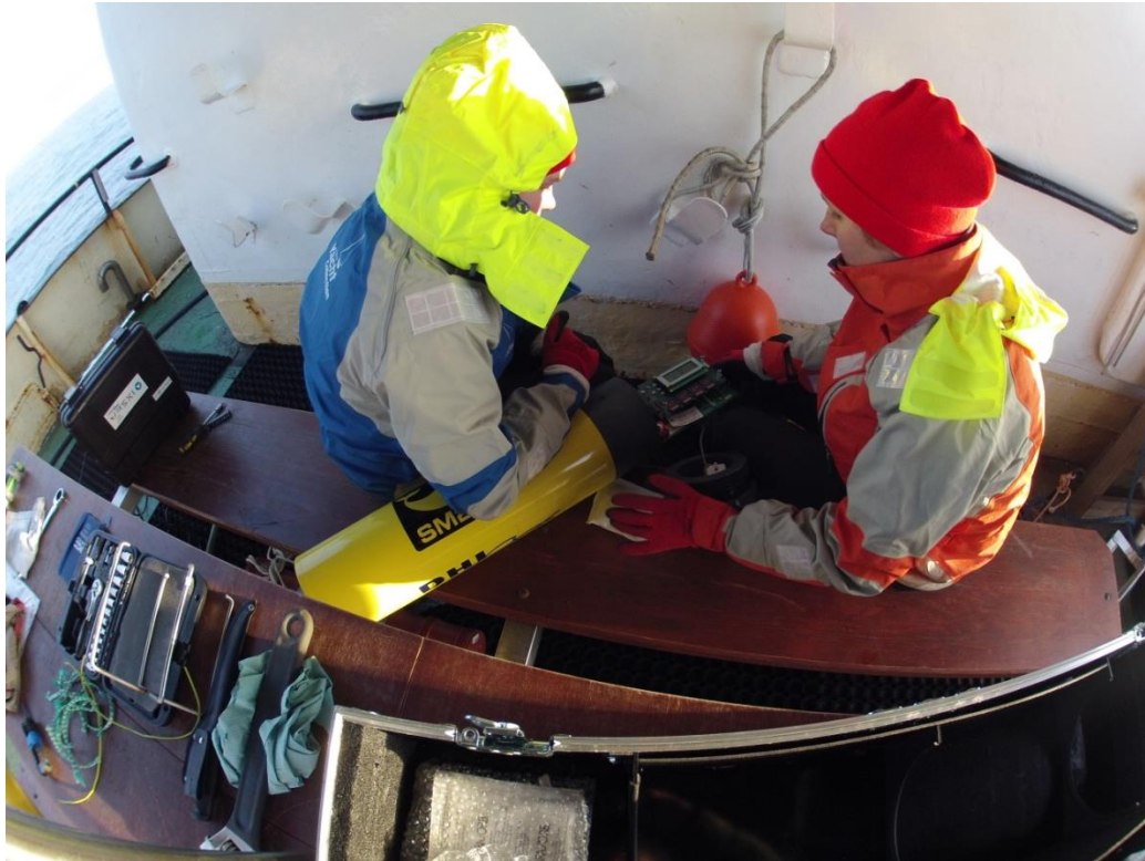
Figure 10 Set up of the acoustic recorder before the deployment
